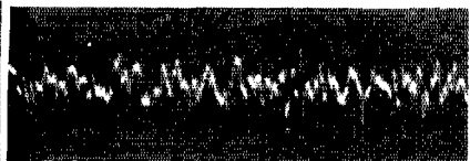
Oscillogram showing noisy performance of other types of resistors.
